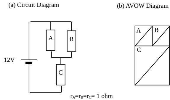
Figure 3 : Equivalent circuit and AVOW diagrams.
