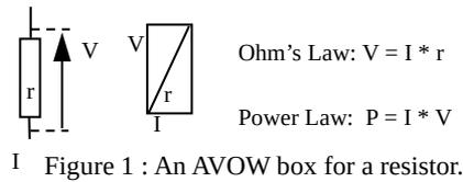
Figure 1 : An AVOW box for a resistor.
